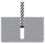
With the correct diameter drill bit, drill a hole to a depth of at least one diameter of the anchor deeper than the required embedment.
