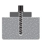
Continue to tighten the anchor until flanged head is firmly seated against fixture.
