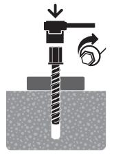
Install with either a socket or cordless impact driver. Apply pressure against the fixing and rotate to engage the first thread
